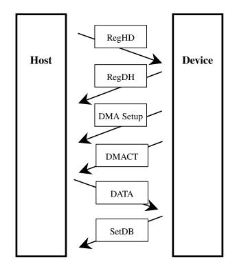
Figure 5.19 WRITE FP DMA QUEUED command protocol
